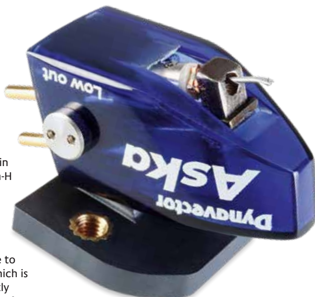
ABOVE: The Aska-L's annealed pole piece/yokes are mounted into a translucent plastic body with lightweight headshell mount. The 6mm alloy cantilever is fitted with an elliptical tip
